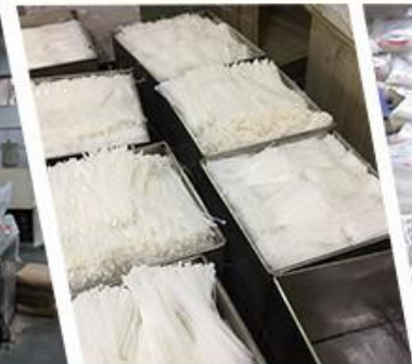
6. Cable Ties After Injection
